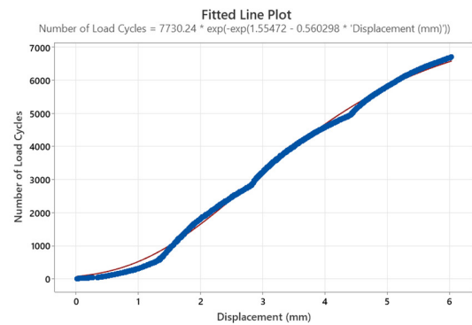
Fig. 12. Overfitted non-linear function of load cycle and displacement in the fatigue shear test of HP at 60°C.
