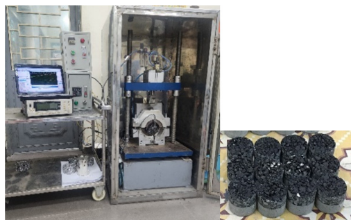
Fig. 4. Fatigue shear test device and specimens.
