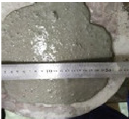
Fig. 1. Flowability test of AHPC.
