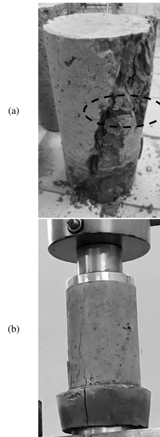
Fig. 3. Failure modes: (a) Damaged column, (b) damaged column rehabilitated by AHPC with underwater concreting.
