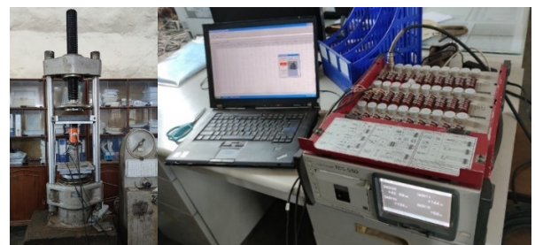
Fig. 8. Determining the elastic modulus of UHPC material (compressing test and laboratory instruments).
