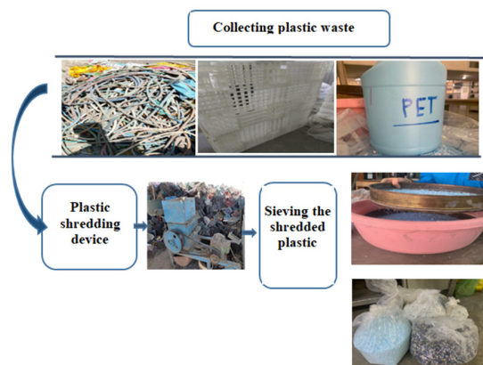
Fig. 2. Preparing process of plastic waste.
