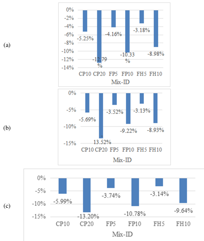
Fig. 6. Variation percentage in compressive strength of the RCC blends after 28 days for (a) water curing, (b) water spraying, (c) coating material.
