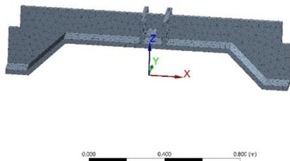
Fig. 10. Modified beam mesh.
