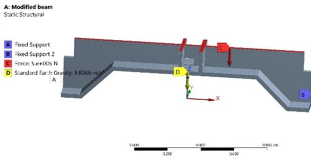
Fig. 11. Loads and boundary conditions for modified beam.
