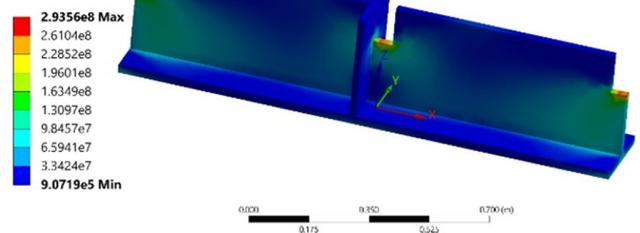
Fig. 9. Von Mises stress distribution for the unmodified beam.
