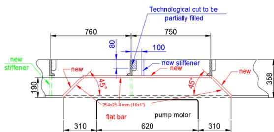
Fig. 6. Constructive solution (modified beam).
