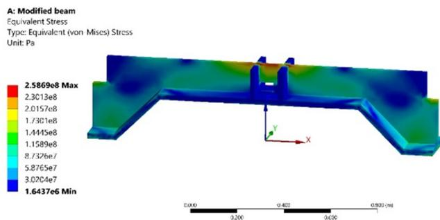
Fig. 12. Von Mises stress distribution for the modified beam.
