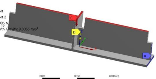
Fig. 8. Loads and boundary conditions for the unmodified beam.
