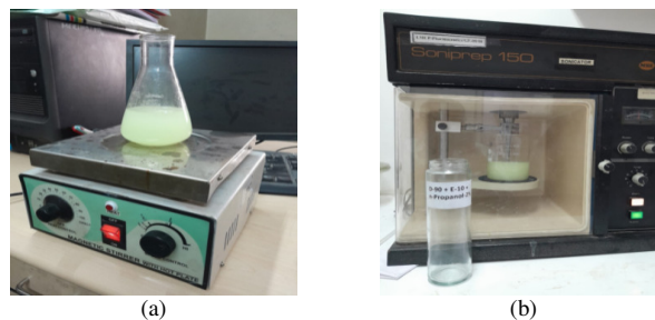
Fig. 3. Experiment work on the magnetic stirrer and probe ultrasonicator.
