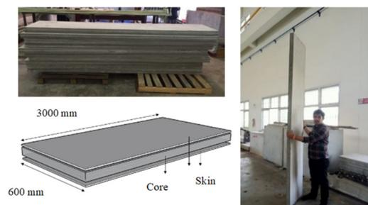
Fig. 1. Prefabricated sandwich panels.
