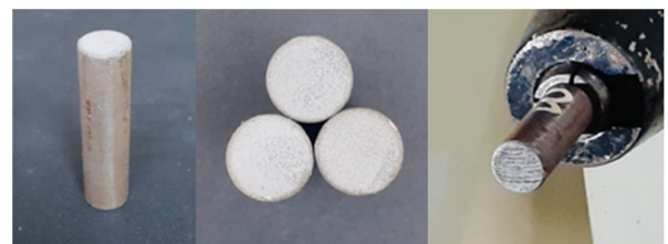
Fig. 2. The test sample after HVOF coating.
