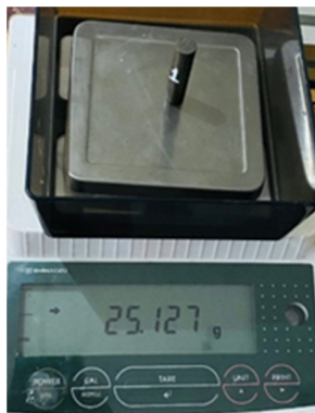
Fig. 4. The electronic scale used to measure the weight of the test samples.
