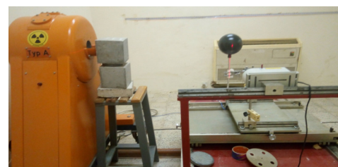
Fig. 3. Experimental setup of the determination of gamma radiation before and after placing the shielding samples.
