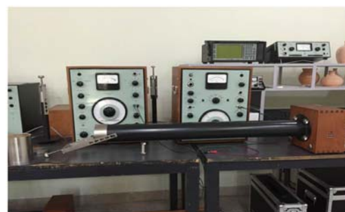
Fig. 3. Measuring instrument for sound absorption.
