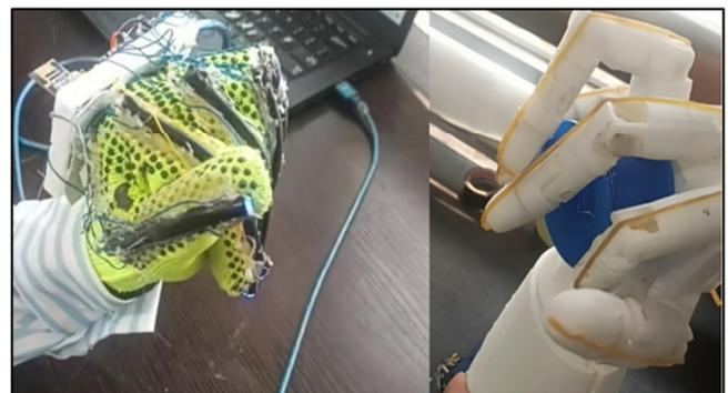
Fig. 13. The robotic hand picking up an object in a manner that closely resembles the human hand.
