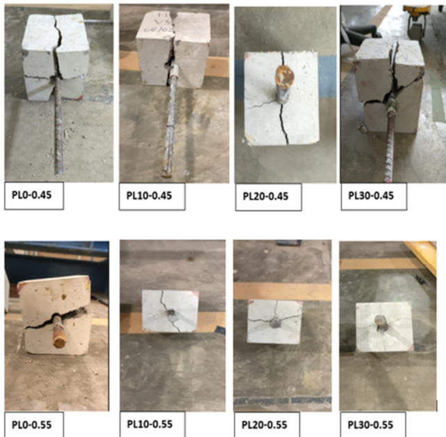
Fig. 7. Failure mode of sample.
