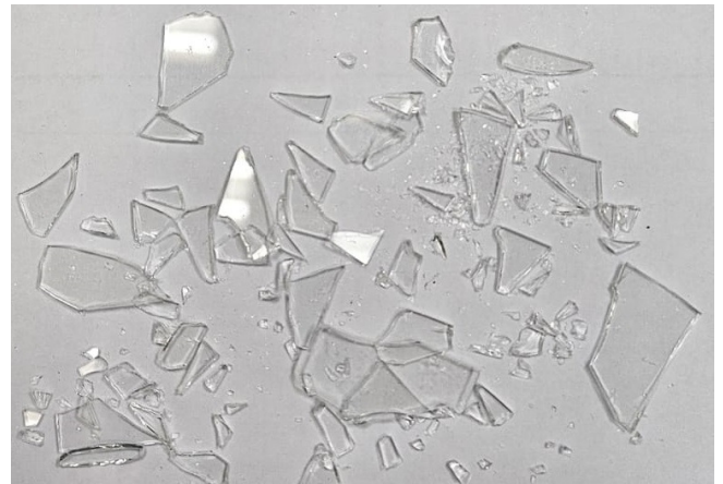
Fig. 1. View of a broken glass slide used to cover the end face of the optical fiber.
