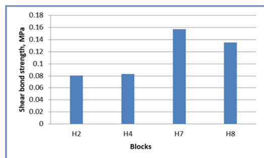
Fig. 13. Effect of hollow shape on shear bond strength.
