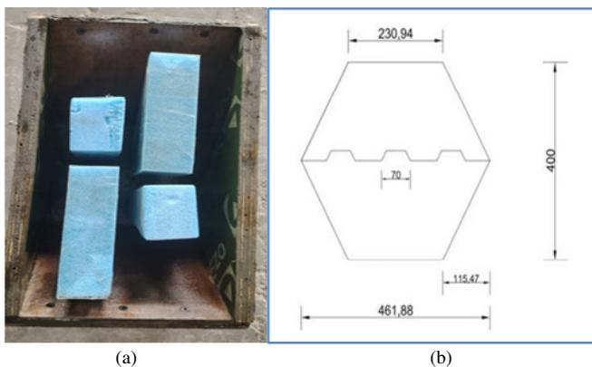
Fig. 7. (a) Hexagonal molds, (b) dimension of hexagonal blocks.
