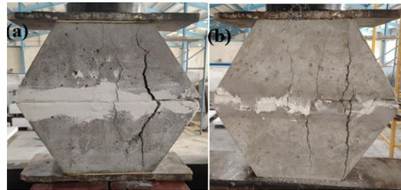
Fig. 20. Failure mode for stacked hexagonal blocks (a) without interlocking, (b) with interlocking.
