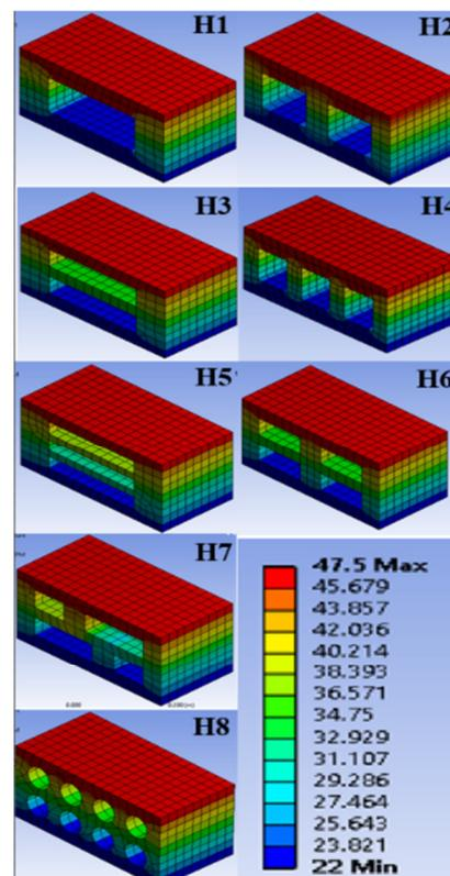
Fig. 3. Temperature distribution for block samples.
