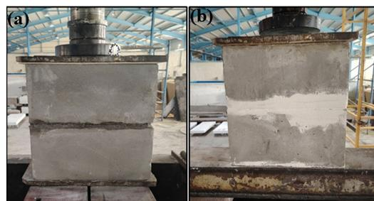
Fig. 16. Compression test for stacked block units (a) cuboid blocks with mortar joint material, B1, (b) cuboid blocks with bonding material, B2.
