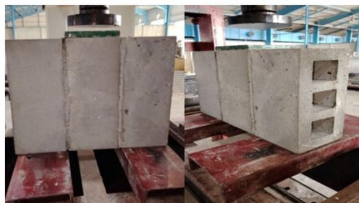
Fig. 9. Shear bond strength test for cuboid blocks.
