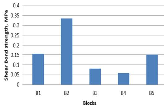
Fig. 21. Bond shear strength results.
