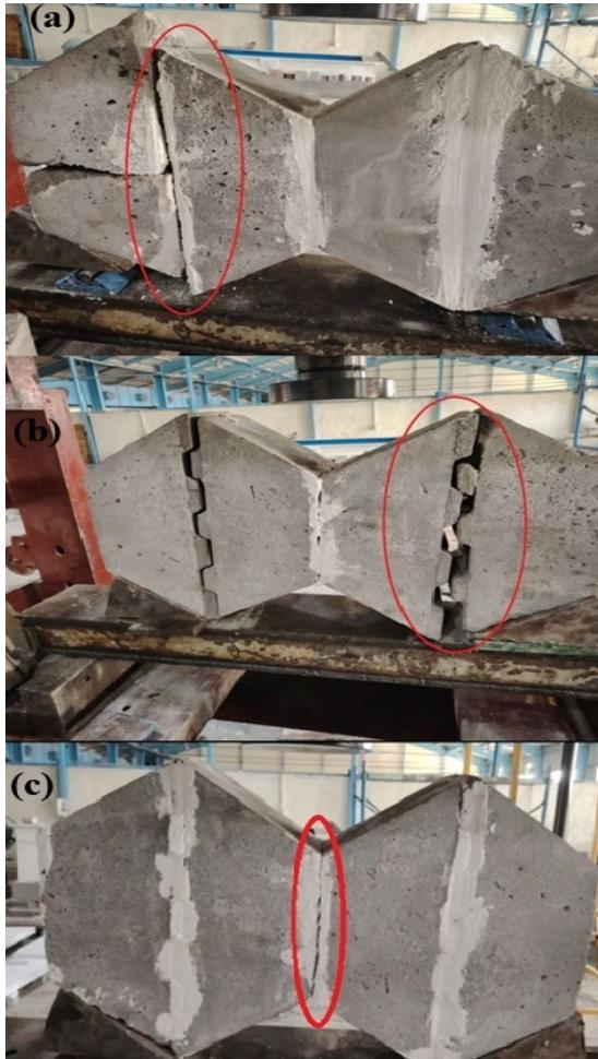
Fig. 23. Failure modes of stacked hexagonal blocks (a) without interlocking and using M2 joint materials, (b) with interlocking and not using a joint material, (c) with interlocking and using M2 joint material.
