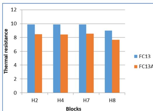
Fig. 15. Thermal resistance of foamed concrete blocks.
