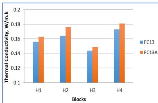
Fig. 14. Thermal conductivity of foamed concrete blocks.
