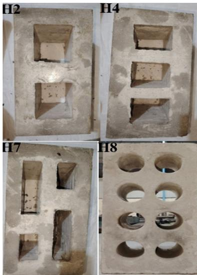
Fig. 6. Hollow foamed concrete blocks.
