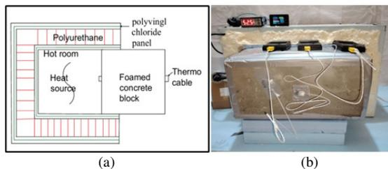
Fig. 10. (a) Locally made thermal conductivity testing device, (b) block unit during thermal conductivity test.
