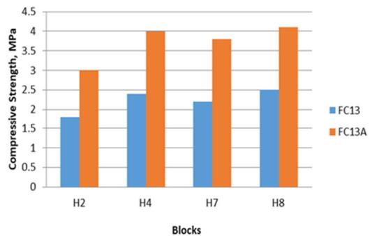
Fig. 12. Compressive strength of hollow foamed concrete blocks made with different hole shapes.
