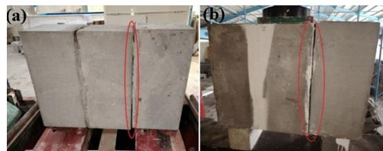
Fig. 22. Failure modes of stacked cuboid blocks (a) M1 joint materials, (b) M2 joint material.
