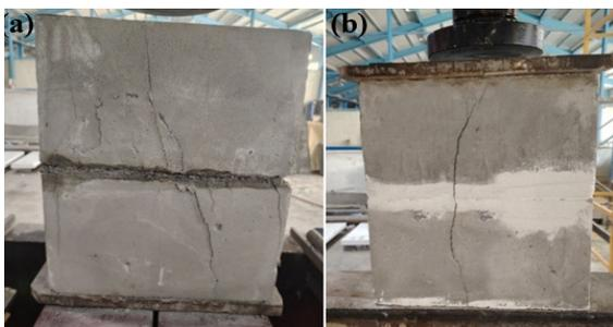
Fig. 19. Failure mode for block, (a) mortar joint material, (b) bonding adhesive material.
