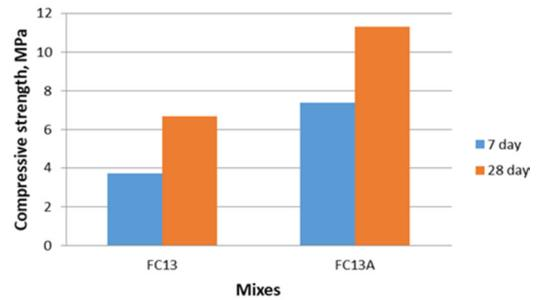
Fig. 11. Compressive strength of investigated foamed concrete mixes.
