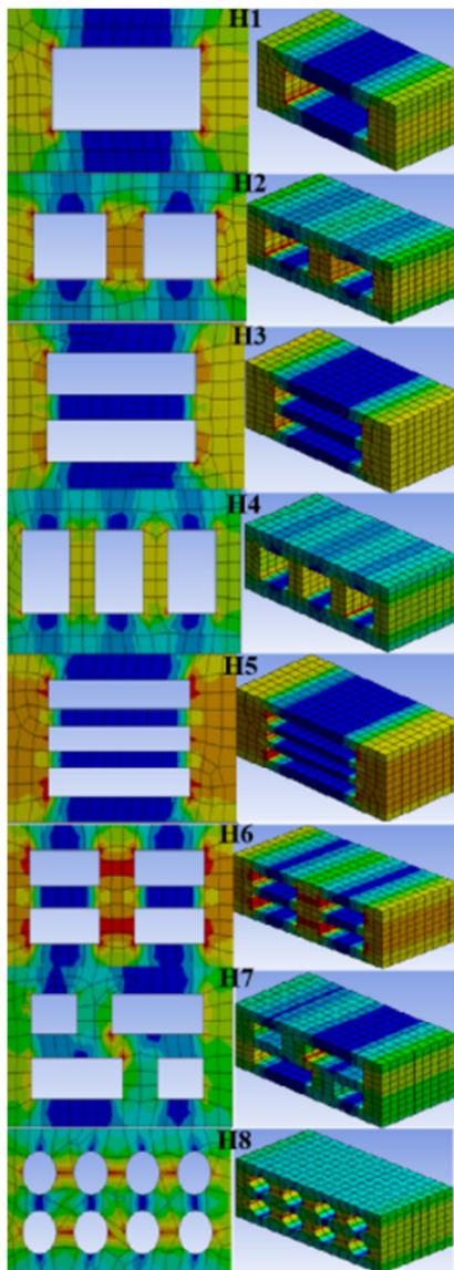
Fig. 2. Heat flow distribution.
