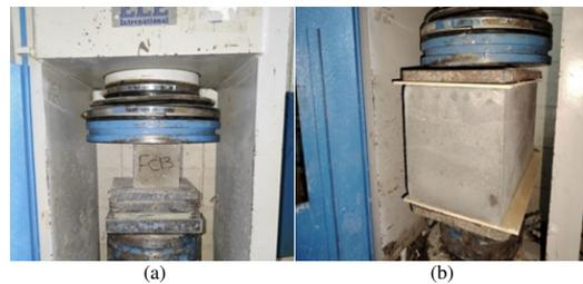
Fig. 8. (a) Compressive strength of sample, (b) compressive strength of hollow concrete block.
