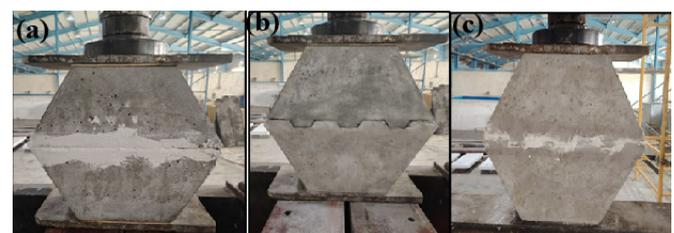
Fig. 17. Compression test for stacked block units (a) Hexagonal blocks with bonding material, B3, (b) hexagonal blocks with mechanical bonding, B4, (c) mechanical bonding techniques with bonding material, B5.
