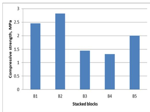
Fig. 18. Compressive strength of stacked blocks.
