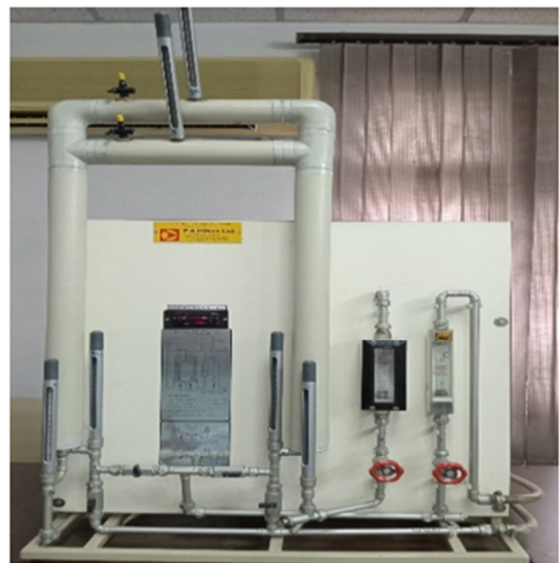
Fig. 1. U-bend concentric tube heat exchanger H900.
