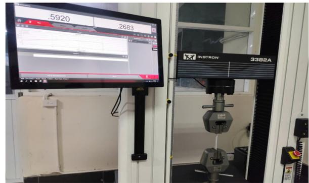
Fig. 3. Picture of the tensile testing process for the PLA specimen..
