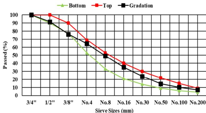
Fig. 3. Gradation of AC-WC mixture.
