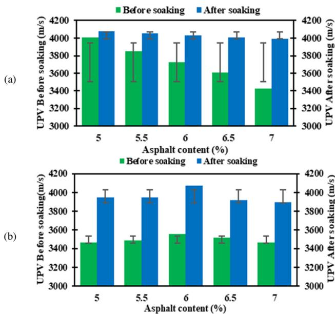
Fig. 14. UPV before and after immersion of the mixtures containing fine aggregates and filler produced through (a) RB waste and (b) SD.
