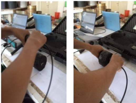
Fig. 5. Device used to implement the UPV method.
