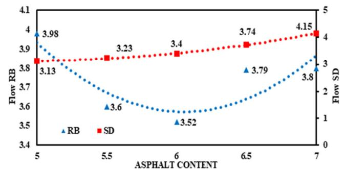
Fig. 7. Flow of RB waste and SD.
