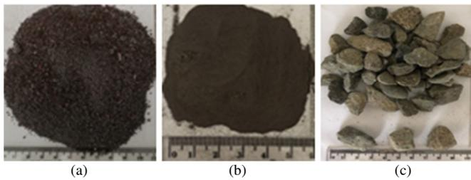
Fig. 2. (a) Filler RB waste, (b) fine aggregate RB waste, and (c) coarse aggregate RB waste.
