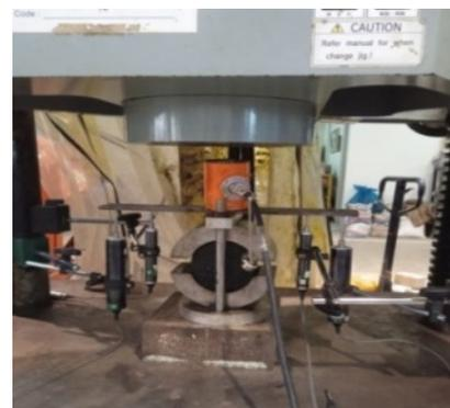
Fig. 4. Marshall apparatus utilized for this study.
