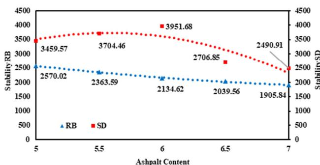
Fig. 6. Stability of RB waste and SD.
