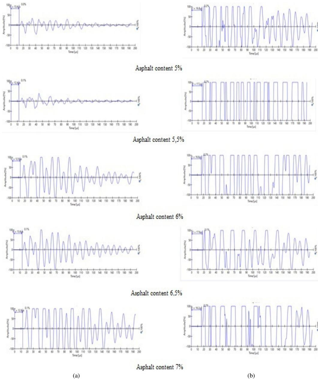
Fig. 13. Ultrasonic wave patterns of the mixtures containing fine aggregates and filler produced through (a) RB waste and (b) SD.
