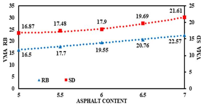
Fig. 10. VMA of RB waste and SD.
