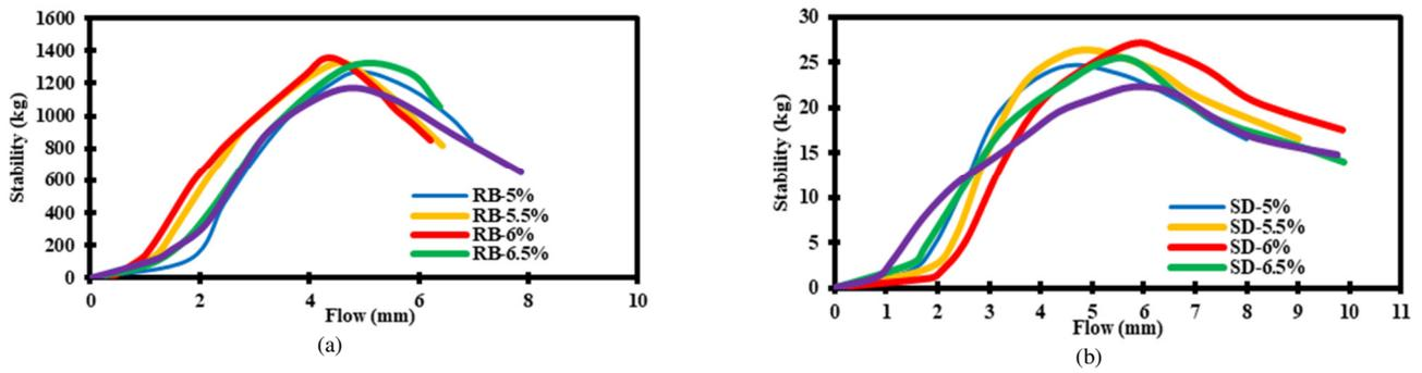
Fig. 12. Correlation between stability and flow of the mixtures containing fine aggregates and filler produced through (a) RB waste and (b) SD.
