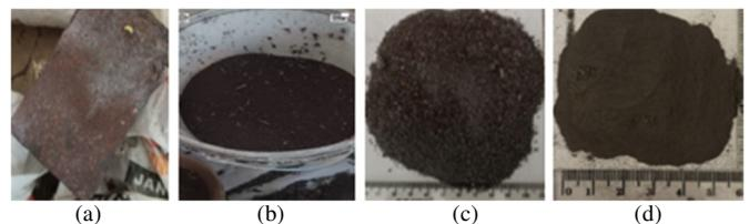
Fig. 1. (a) Processing of raw RB waste in block form, (b) crushing and sifting of the block form with a hammer, (c) fine aggregates passed through sieve No. 4, and (d) filler passed through sieve No. 200.
