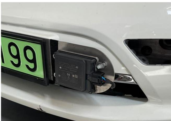
Fig. 2. The installed Continental ARS 408-21 long-range radar.
