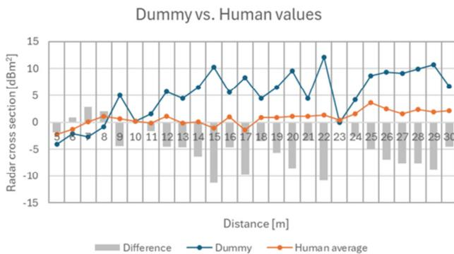
Fig. 4. Average RCS values and differences between dummy and humans.
