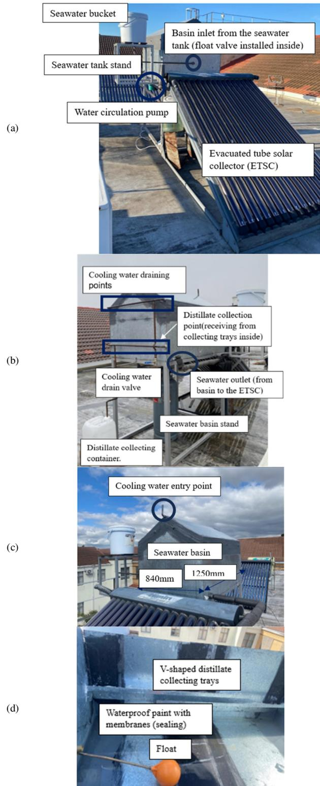
Fig. 1. Solar still (a) overview including the ESTC, (b) seawater piping, (c) basin measurements, (d) inside the water basin.
