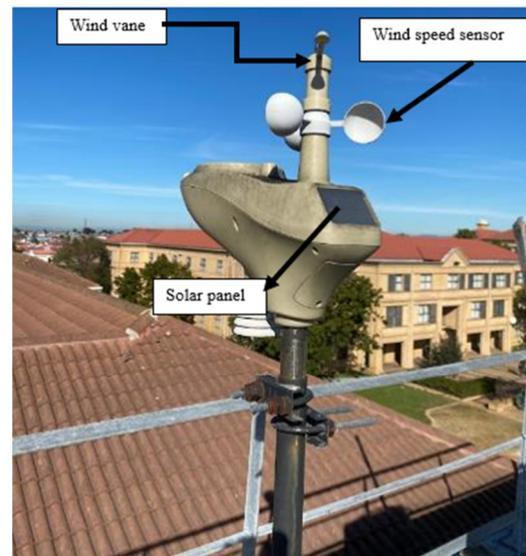
Fig. 2. HP2000 wireless weather station.
