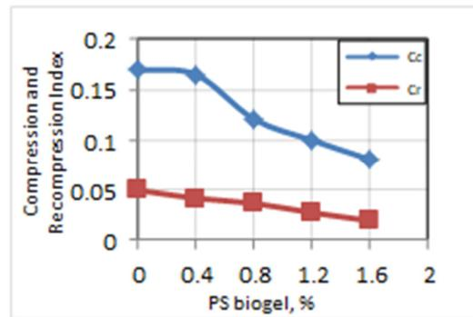
Fig. 9. Variation in  $C_c$  and  $C_r$  with different percentages of PS biogel.
