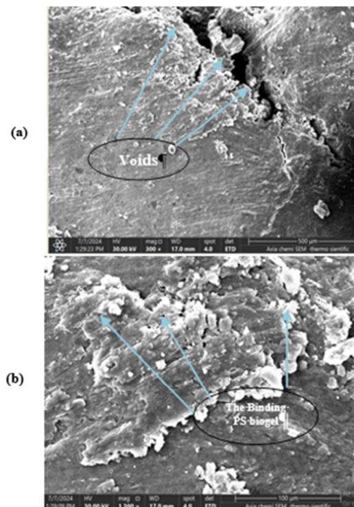
Fig. 14. SEM test of (a) untreated sample and (b) treated sample with 0.8% PS gel.
