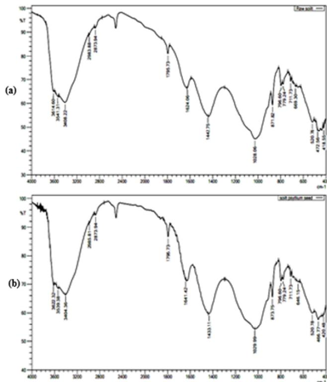
Fig. 15. FTIR analysis for (a) prepared expansive soil and (b) prepared expansive soil with 0.8% PS biogel.
