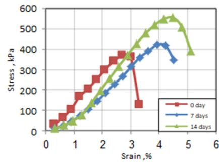
Fig. 13. Stress-Strain relationship for prepared expansive soil treated with 0.8% PS biogel at different curing periods.
