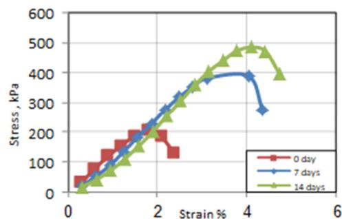
Fig. 12. Stress-Strain relationship for prepared expansive soil at different curing periods.
