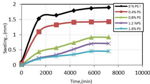
Fig. 7. Relationship between swelling and time for prepared expansive soil with varying percentages of PS biogel.
