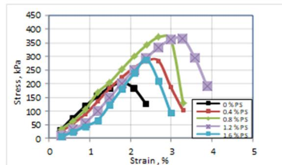
Fig. 10. Stress-Strain relationship for prepared expansive soil with different percentages of PS biogel.
