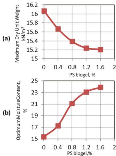
Fig. 4. Variation in (a) maximum dry unit weight (kN/m<sup>3</sup>) and (b) OMC (%), with different percentages of PS biogel.
