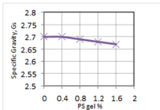
Fig. 5. Variation in G<sub>s</sub> of expansive soil with different percentages of PS biogel.
