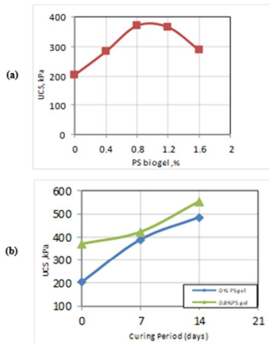
Fig. 11. UC of soil treated with PS biogel at (a) different percentages and (b) different curing periods.
