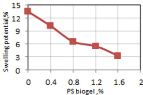
Fig. 8. Variation in swelling potential % of expansive soil with different percentages of PS biogel.
