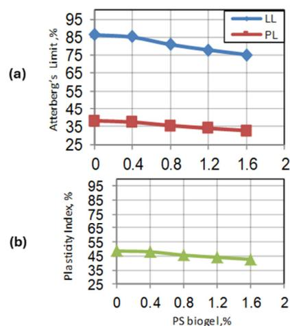
Fig. 6. Variation in (a) Atterberg's limits (%) and (b) PI (%), with different percentages of PS biogel.
