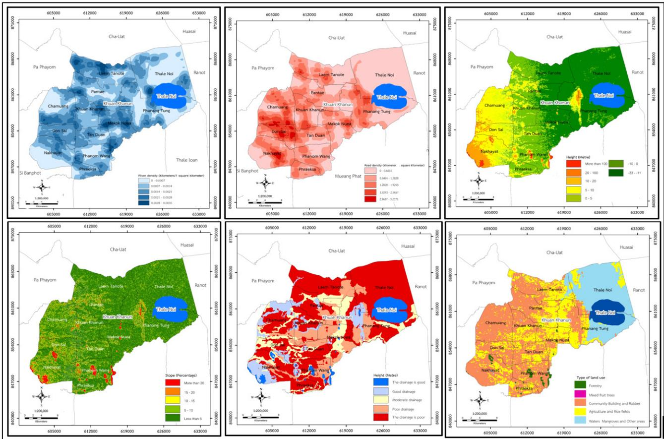
Fig. 3. Input maps for flood hazard assessment including (from left to right and from up to down): (a) river density, (b) road density, (c) slope, (d) elevation, (e) soil drainage, and (f) land use.
