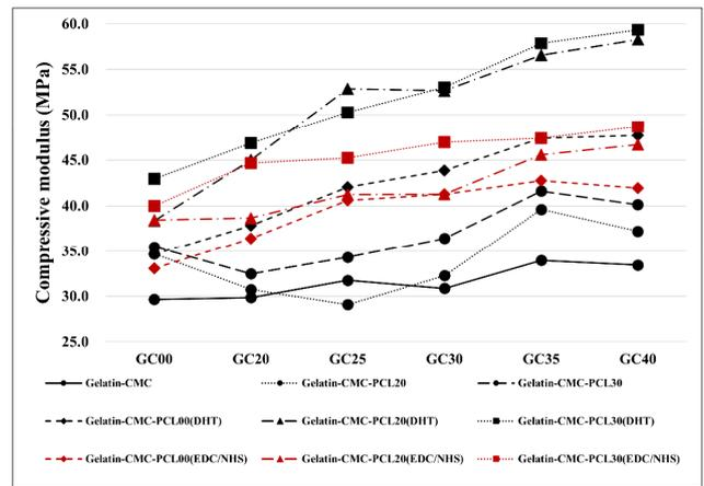
Fig. 6. Average compressive modulus (MPa) at various mixing proportions of gelatin-CMC-PCL scaffolds of non-crosslink, crosslinked by DHT and EDC/NHS.
