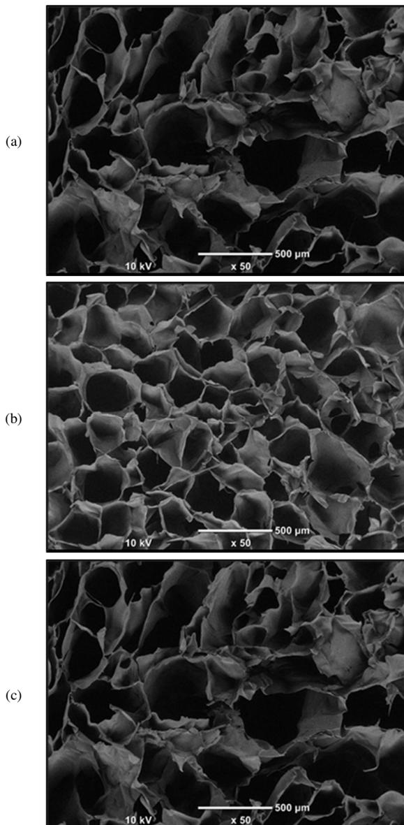
Fig. 3. SEM images of gelatin-CMC-PCL scaffolds: (a) GC40P30, (b) GC40P30 (crosslinked by DHT), (c) GC40P30 (crosslinked by EDC/NHS).
