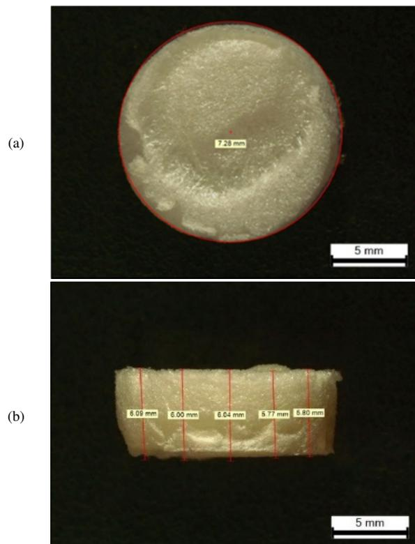
Fig. 2. 3D gelatin-CMC-PCL scaffold: (a) front view and (b) side view.
