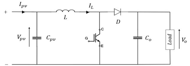
Fig. 4. The used boost DC-DC converter circuit.
