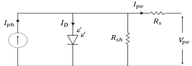
Fig. 1. Schematic representation of the PV cell.
