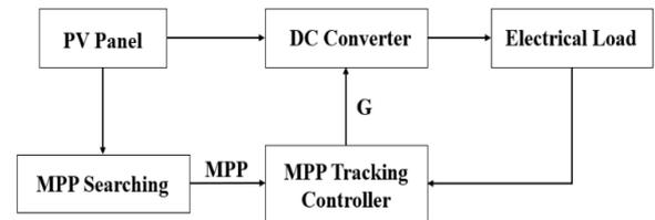
Fig. 6. The block diagram of dual-loop control scheme.
