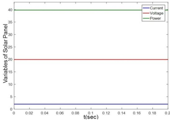
Fig. 8. Power, voltage, and current of the PV panel without any MPPT method under STC.
