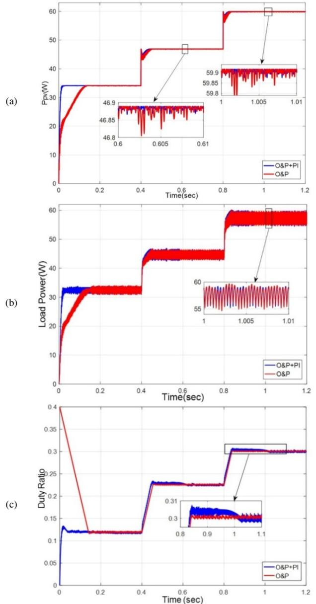
Fig. 10. Dynamic response of the proposed MPPT schemes under variable irradiation conditions: (a) power of PV panel, (b) load power, and (c) duty ratio.
