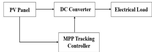
Fig. 5. A typical photovoltaic power source.
