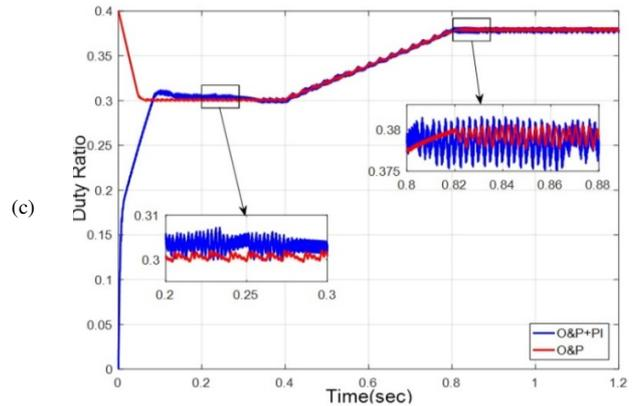
Fig. 12. Dynamic response of the proposed MPPT schemes under variable temperature conditions: (a) power of PV panel, (b) load power, and (c) duty ratio.
