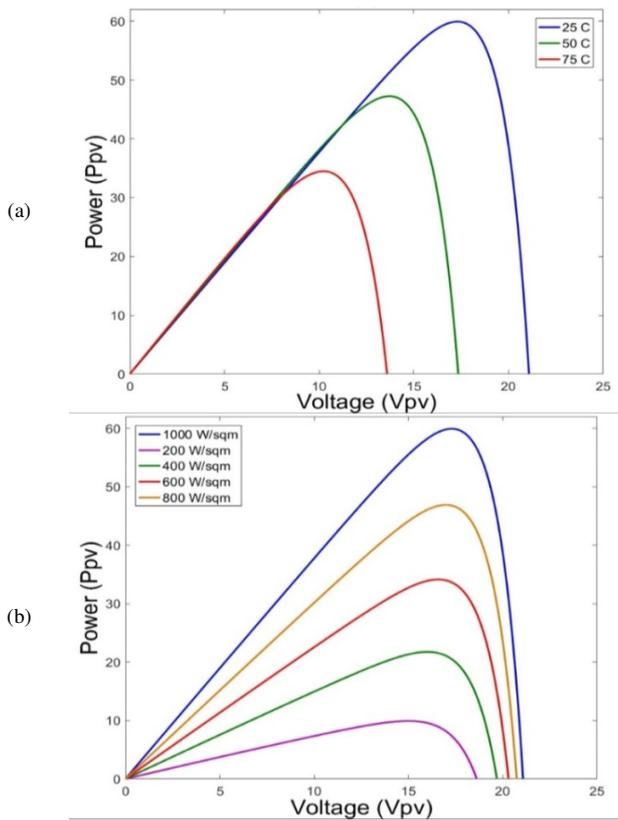
Fig. 3. P-V characteristic with (a) variable temperature, (b) variable irradiance.
