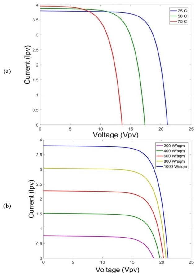
Fig. 2. I-V characteristic with (a) variable temperature, (b) variable irradiance.
