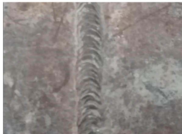
Fig. 2. Visualization of the shape of the welded joint.
