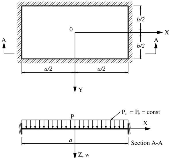
Fig. 2. Rectangular plate subjected to uniform load.
