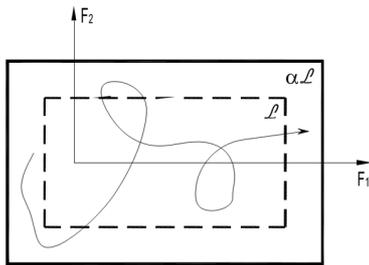
Fig. 1. Convex load domain  $\mathcal{L}$  for two forces.
