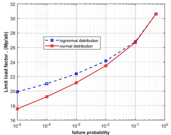
Fig. 4. Limit load factor over failure probability for simply plate ( $\times \frac{m_p}{ab}$ ).
