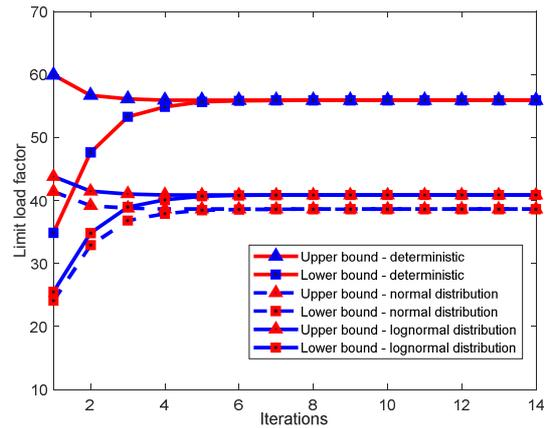
Fig. 3. Convergence of the limit load factors ( $\times \frac{m_p}{ab}$ ).
