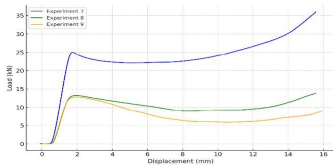
Fig. 5. Load-displacement curves for dodecahedron structure.
