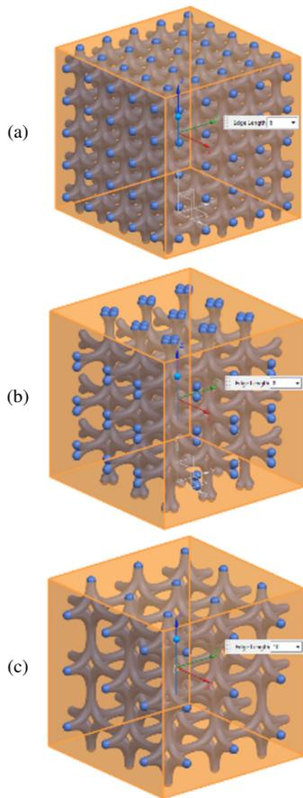
Fig. 1. CAD models of 3D-printed structures: (a) octapeak, (b) hexstar, (c) dodecahedron.
