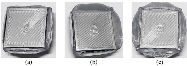
Fig. 2. Physical appearance of 3D-printed structures after compression testing: (a) octapeak, (b) hexstar, (c) dodecahedron.
