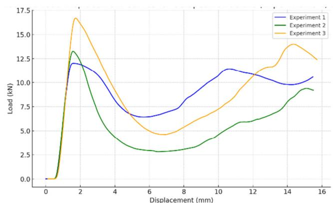
Fig. 3. Load-displacement curves for octapeak structure.
