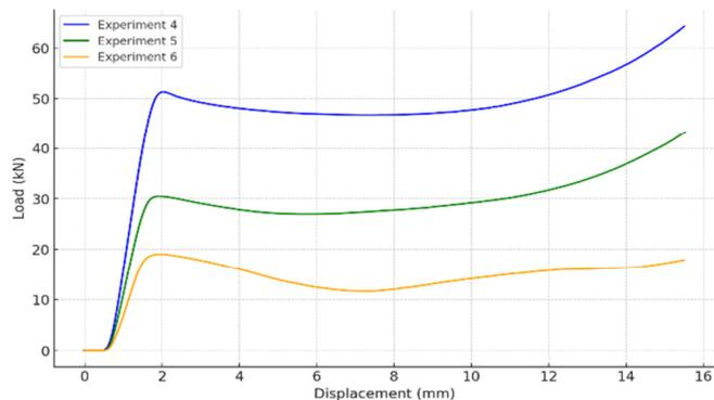
Fig. 4. Load-displacement curves for hexstar structure.
