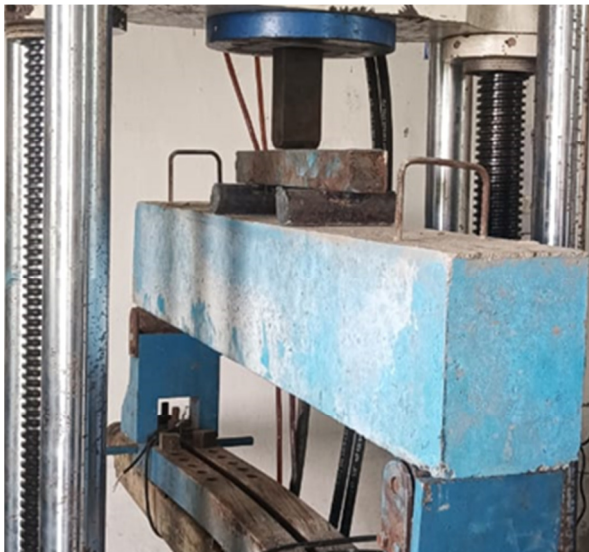
Fig. 5. Flexural strength test.
