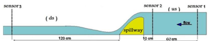
Fig. 5. Representation of the location of water level sensor measurements.
