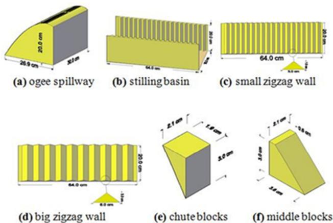
Fig. 4. The dimensioned elements of laboratory models.
