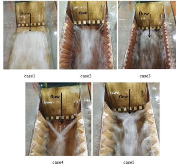
Fig. 7. The flow behavior of water steam in stilling basin for each case.
