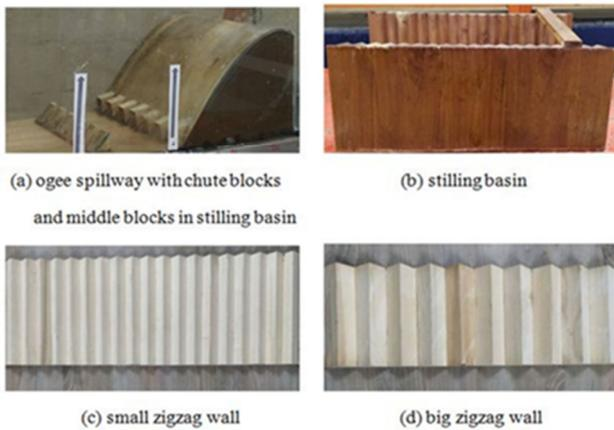
Fig. 3. Laboratory models of (a) the ogee spillway, (b) the stilling basin, (c) the small zigzag wall, and (d) the large zigzag wall.
