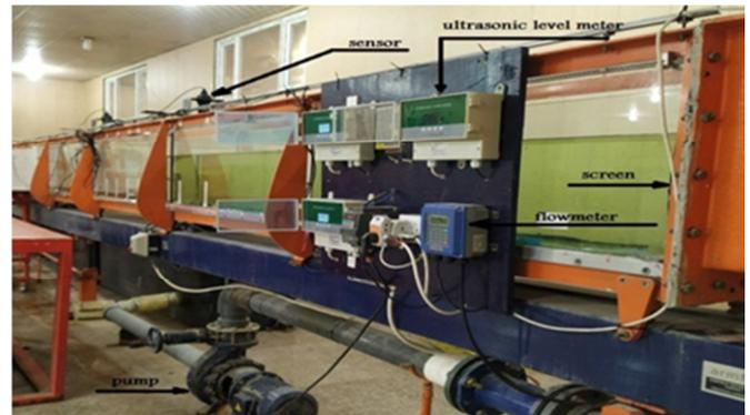
Fig. 1. Experimental setup of laboratory flume.
