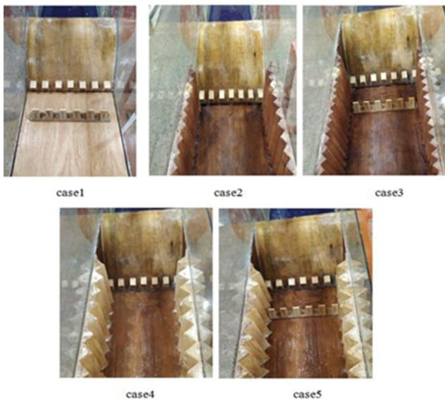
Fig. 2. The five laboratory models of the alternative stilling basin.
