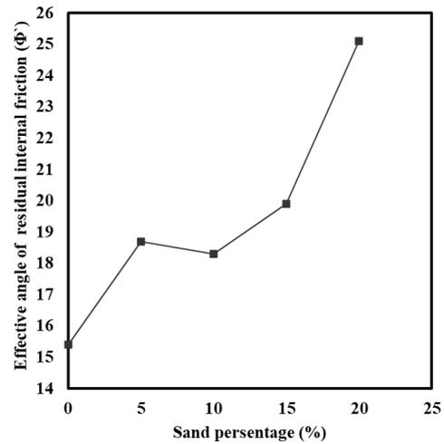
Fig. 8. Variation of residual effective internal friction angle with sand addition in residual shear test.
