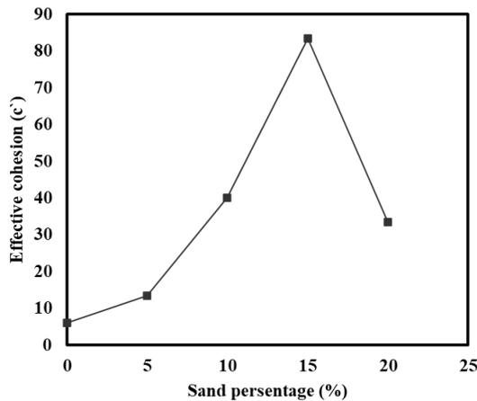
Fig. 6. Variation of effective cohesion with sand addition.
