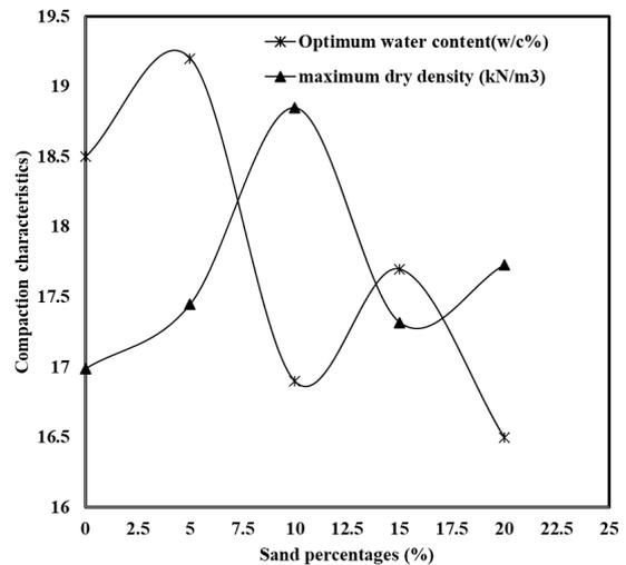
Fig. 3. Variation of compaction characteristics with sand addition.
