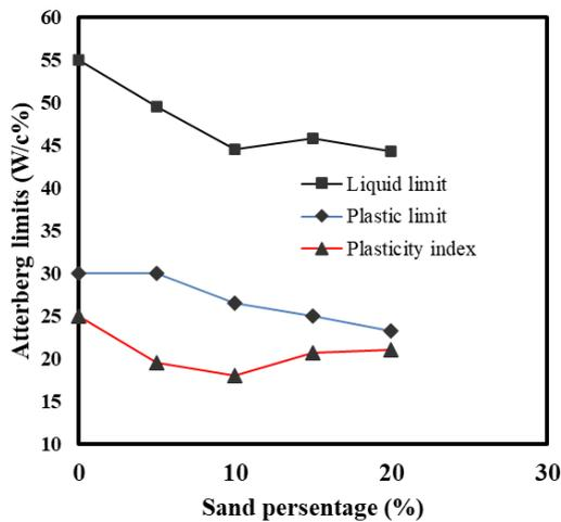
Fig. 1. Variation of Atterberg limits with sand addition.
