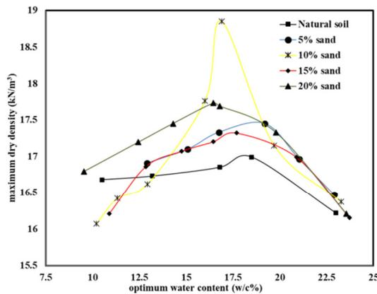
Fig. 2. Compaction characteristics of natural clay and clayey soil-sand mixtures.
