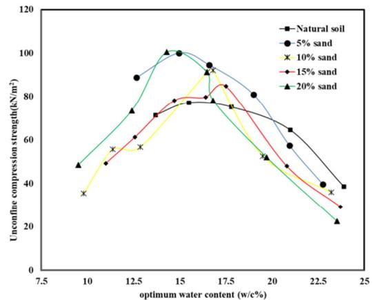
Fig. 4. UCS of natural clay and clayey soil-sand mixtures.
