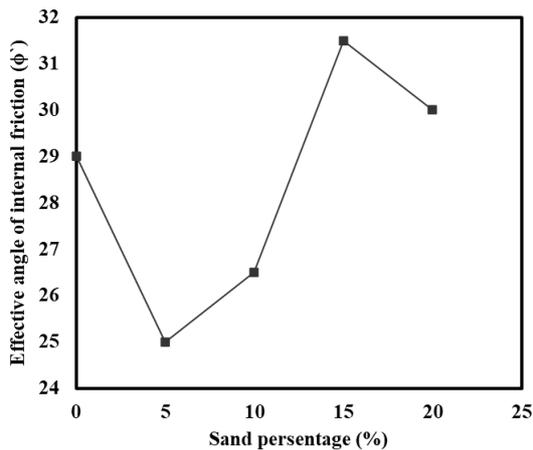
Fig. 7. Variation of effective internal friction angle with sand addition in the direct shear test.
