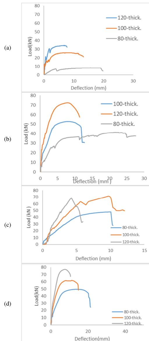
Fig. 8. Effect of thickness on HCS: (a) WC-HCS-A with  $\rho_{min}$ , WC-HCS-B with 2 $\rho_{min}$ , WC-HCS-D with 2 $\rho_{min}$ , (d) NC-HCS-C with 2 $\rho_{min}$ .
