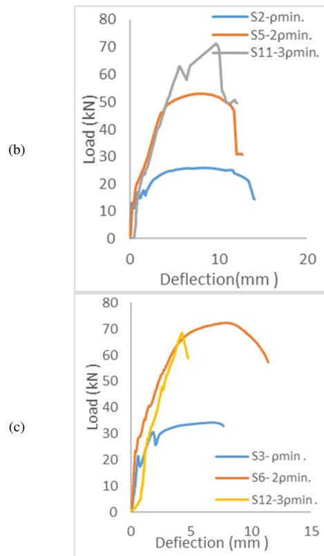
Fig. 9. The effect of reinforcement ratio on the tested WC- HCS: (a) WC- HCS -80 mm, (b) WC- HCS -100 mm, (c) WC- HCS-120 mm.
