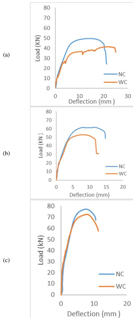
Fig. 10. Effect of concrete type: (a) HCS-80 mm, (b) HCS-100 mm, (c) HCS-120 mm.
