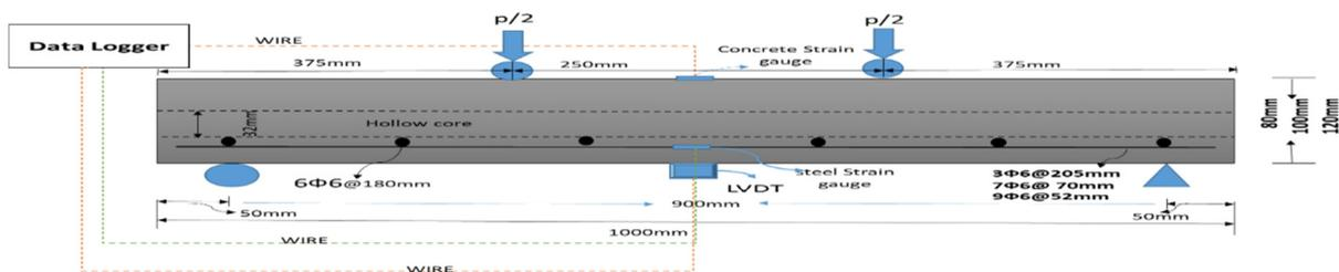
Fig. 2. Details of the slab test.
