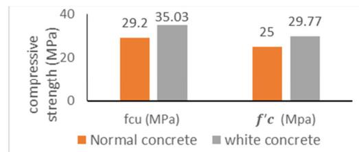
Fig. 5. Compressive strength results.
