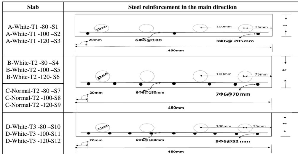
Fig. 3. HCS with steel reinforcement details in the main direction t = 80 mm, 100 mm, 120 mm.
