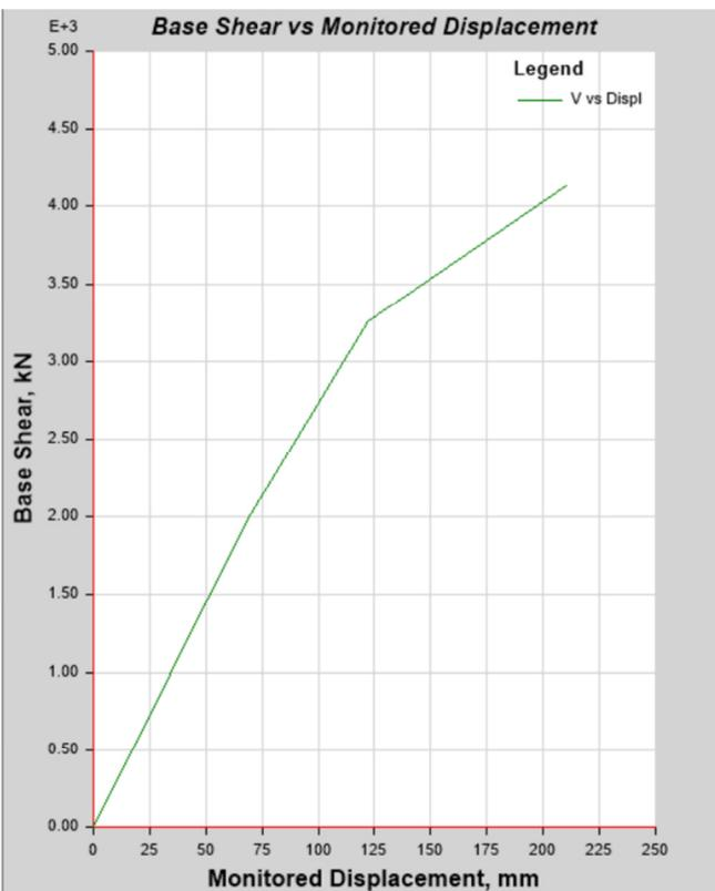
Fig. 9. Y direction capacity curve.
