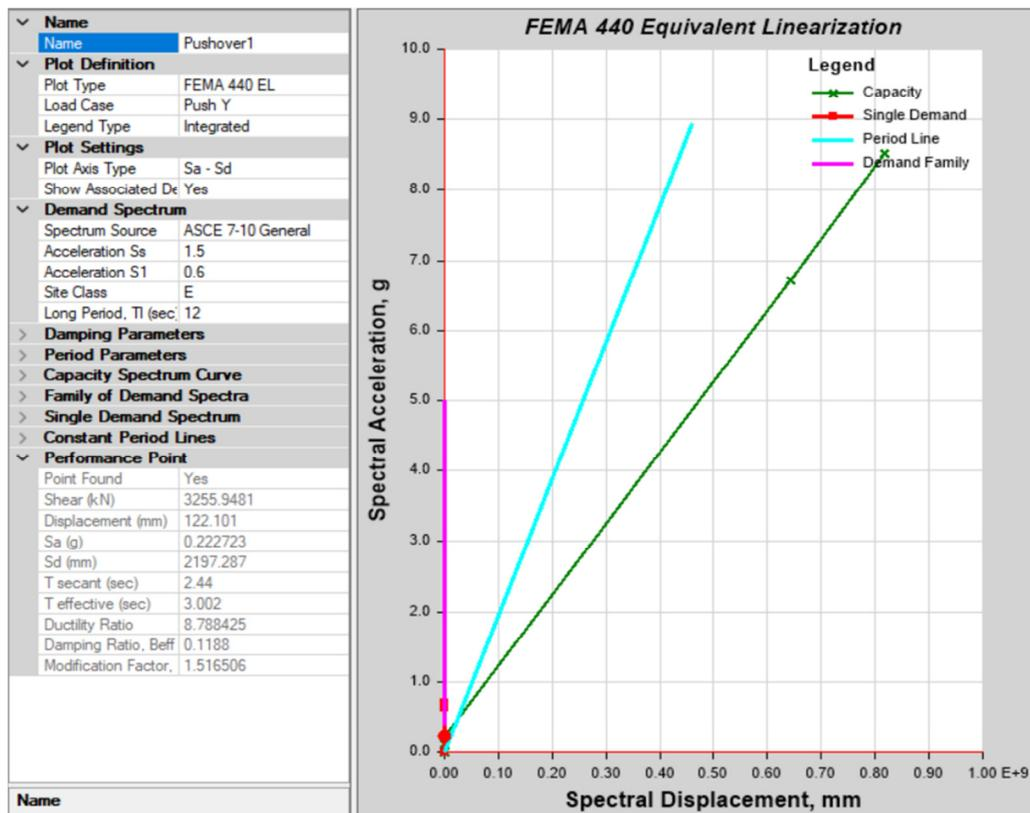
Fig. 13. Performance point FEMA 440 method Y-direction.
