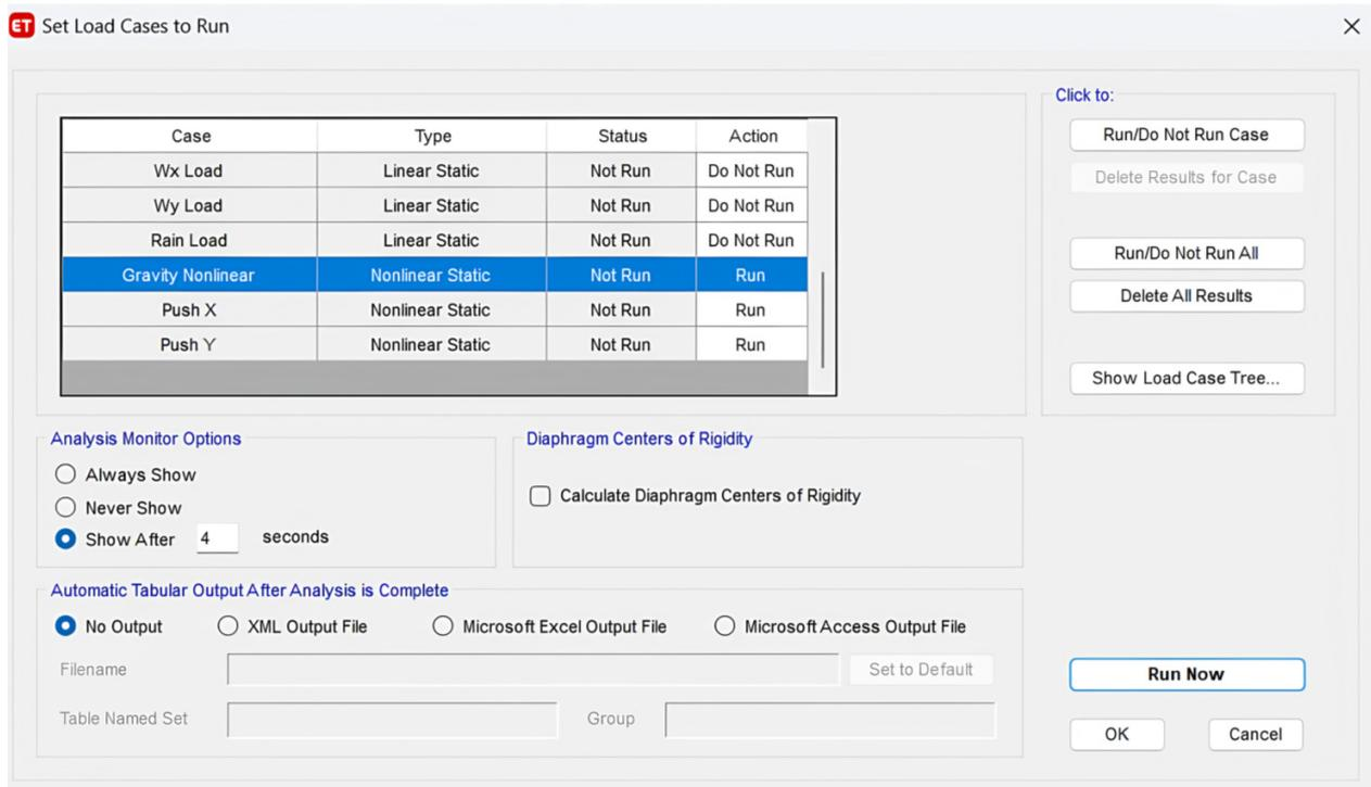
Fig. 7. Setting load cases to run.
