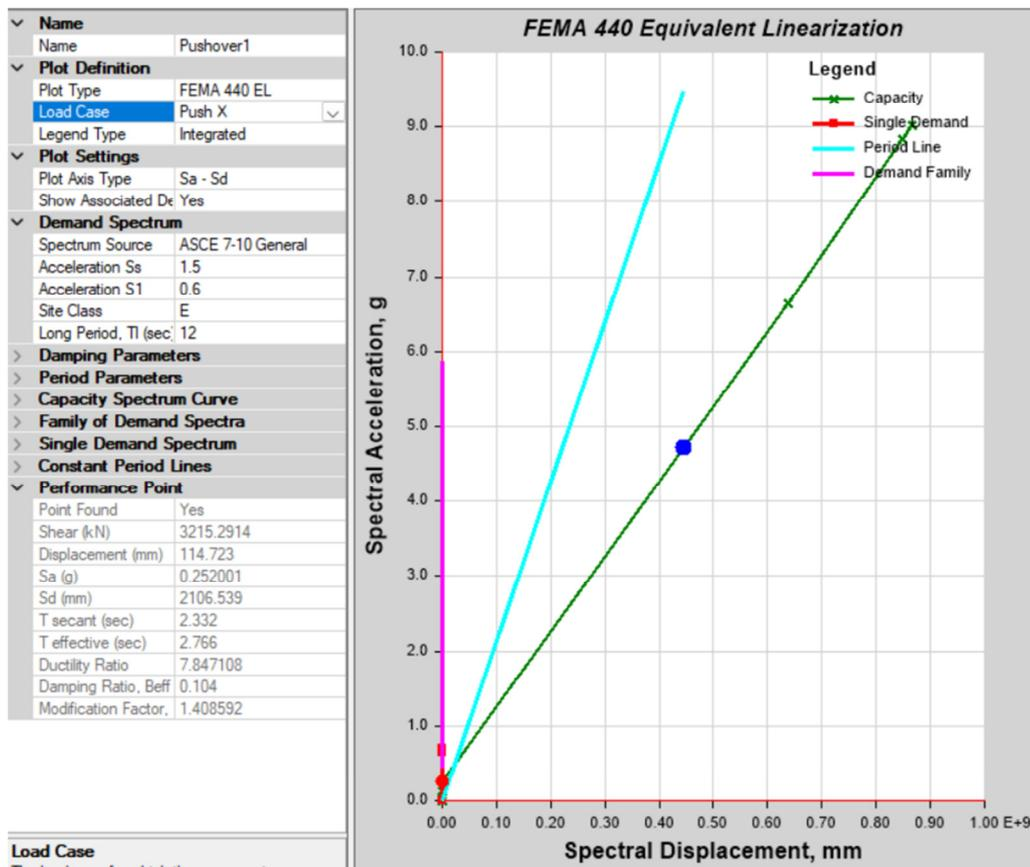
Fig. 12. Performance point FEMA 440 method X-direction.
