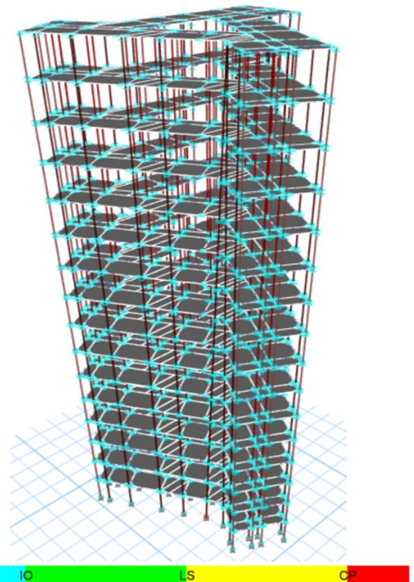
Fig. 11. Plastic joint placement at step 4. Y-direction.
