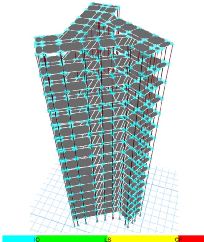
Fig. 10. Plastic joint placement at step 5. X-direction.
