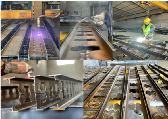
Fig. 8. Process of manufacturing castellated steel beams.
