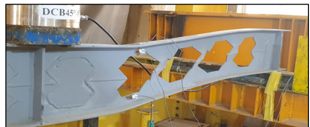
Fig. 16. Mode of failure for CB45°-8.
