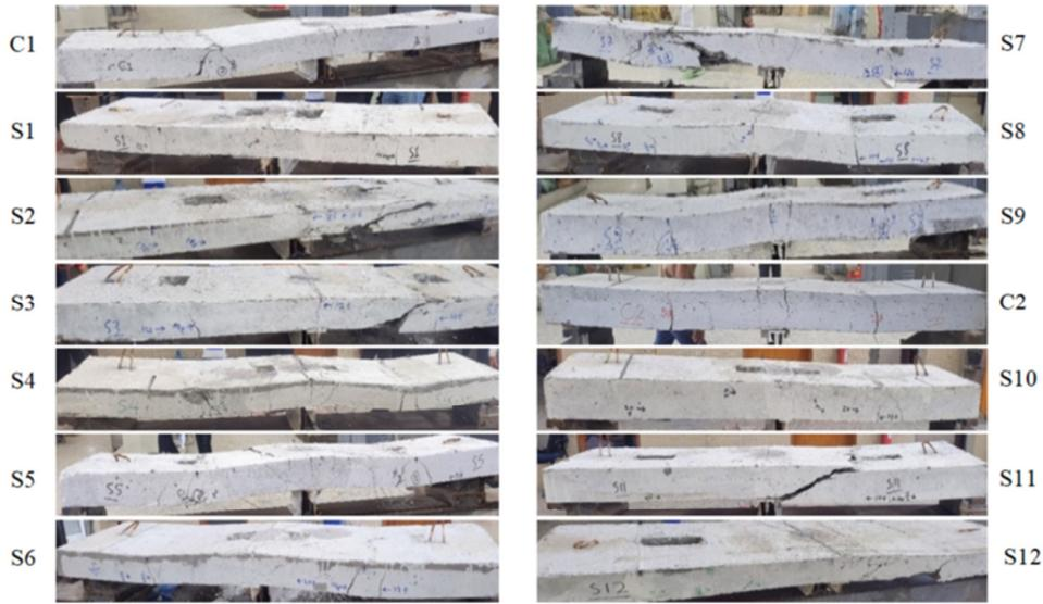
Fig. 4. Failed specimens after test.
