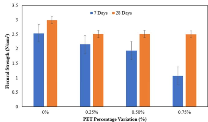
Fig. 10. Flexural strength test results.
