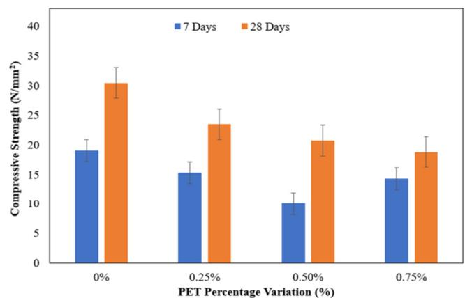
Fig. 9. Compressive strength test results.
