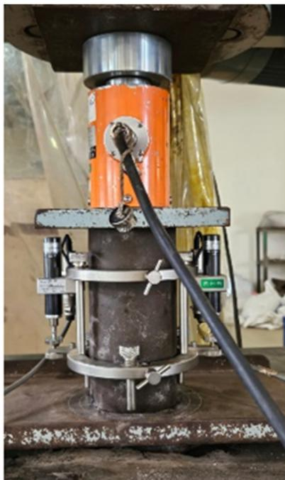
Fig. 6. Compressive strength test.
