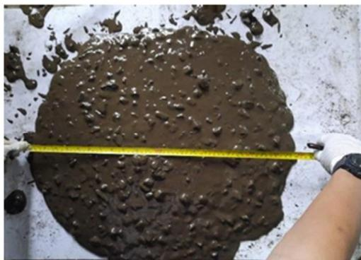
Fig. 5. Slump flow testing.
