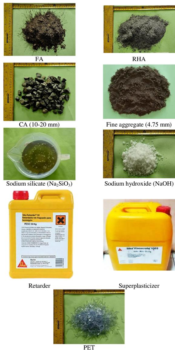
Fig. 3. Materials of geopolymer concrete.
