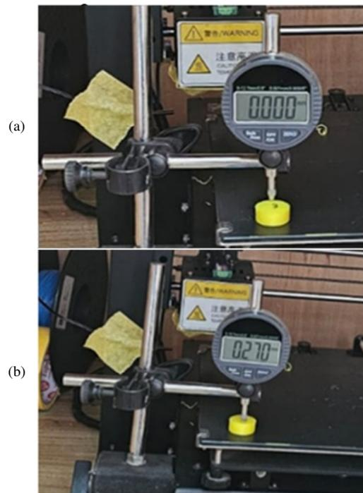
Fig. 8. Measure warping error: (a) set the device to zero, (b) measure the maximum error on sample 1.
