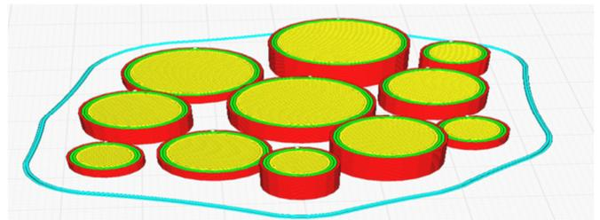
Fig. 5. The cylindrical samples sliced in CURA Slicer software.
