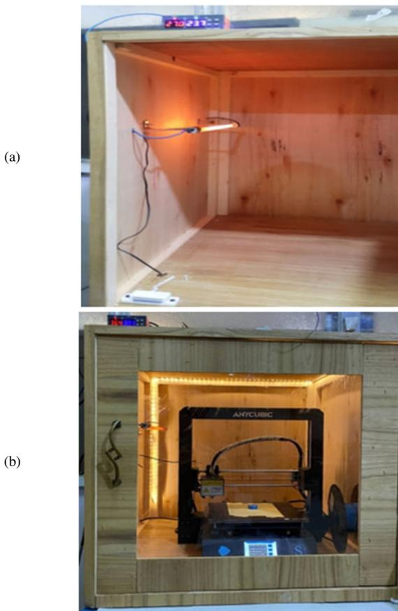
Fig. 6. (a) Heat fixed inside the enclosure, (b) 3D printer inside the enclosure.
