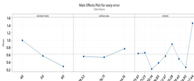
Fig. 9. The main effect of warping error with the range of enclosed temperature, surface area, and volume of nine cylindrical samples.
