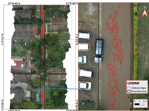
Fig. 8. Edge detection for Innovation-Street road distress condition (lower section of the road).
