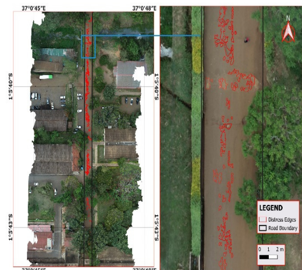
Fig. 7. Edge detection for Innovation-Street road distress condition (upper section of the road).
