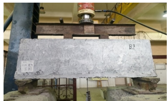
Fig. 4. Test setup of the deep beam specimens.
