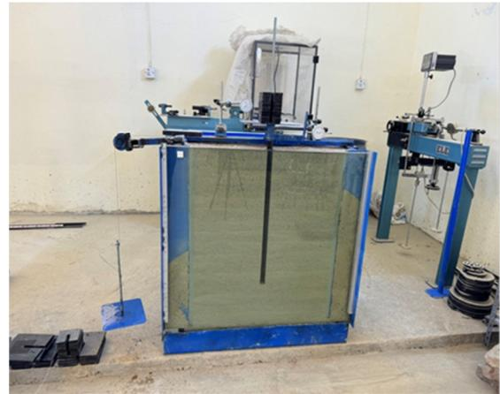
Fig. 4. Vertical load test.
