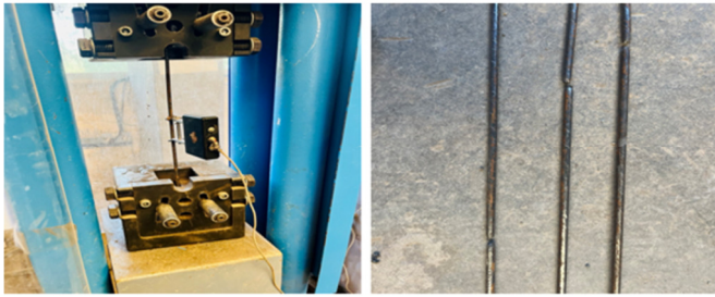
Fig. 2. Tensile test of reinforcements.
