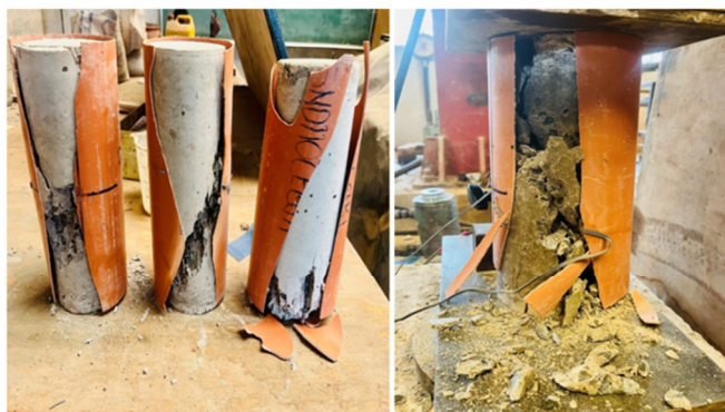
Fig. 14. Brittle shear-type failure mode of exposed specimens.
