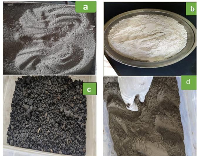
Fig. 1. (a) Expansive soil, (b) WMD, (c) oven dried NP, (d) crushed product of NP.
