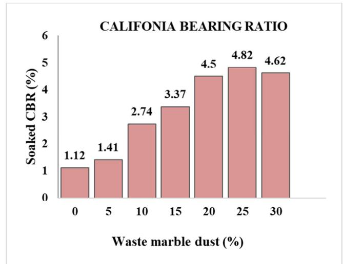
Fig. 10. Soaked CBR of expansive soil treated with WMD.
