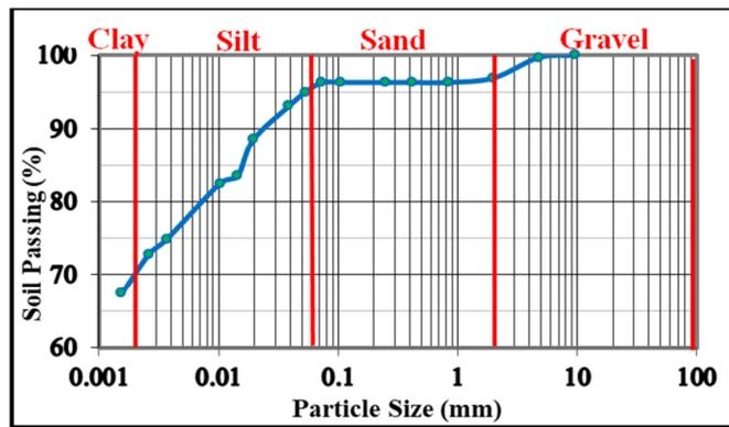
Fig. 3. Particle size distribution curve.
