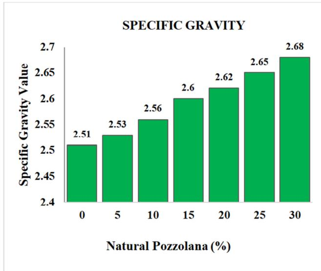
Fig. 8. Change of specific gravity of the expansive soil after mixing with optimum WMD and NP.
