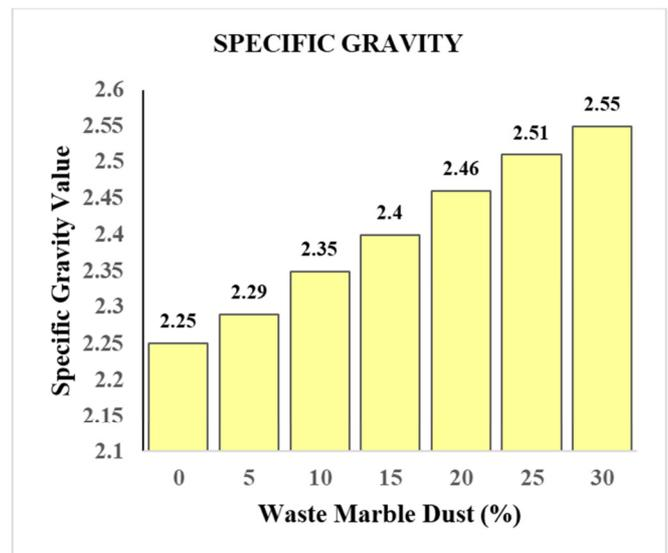
Fig. 6. Change of specific gravity of the expansive soil after mixed with WMD.
