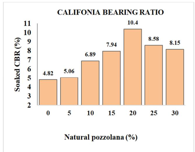
Fig. 11. Soaked CBR of expansive soil treated with optimum WMD and varying NP.
