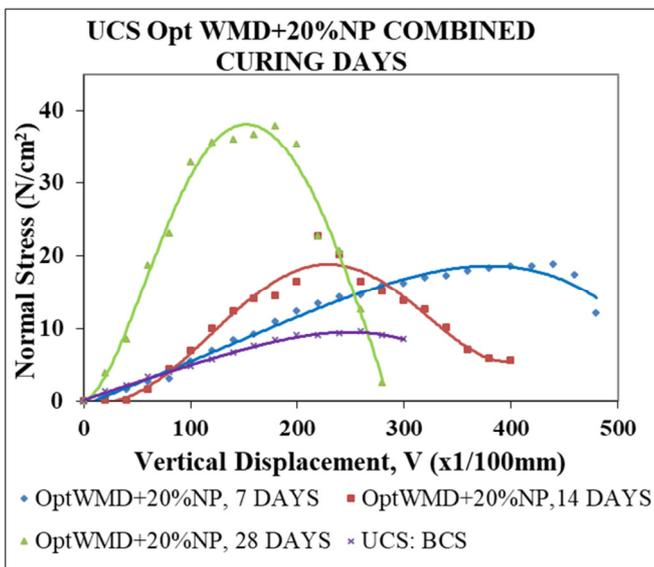
Fig. 13. UCS of expansive soil stabilized with optimum WMD and optimum NP.
