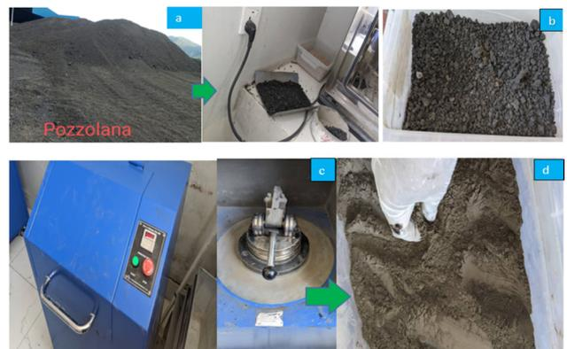
Fig. 2. Treatment and preparation of NP: (a) Collection, (b) oven drying, (c) crushing in vibratory mill, (d) powder.
