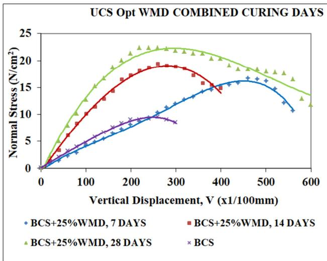
Fig. 12. UCS of expansive soil stabilized by optimum WMD.
