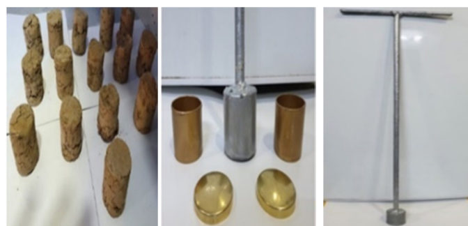
Fig. 2. Soil samples and the core sampler for measuring soil bulk density.
