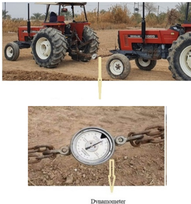
Fig. 3. Dynamometer to measure draft force.
