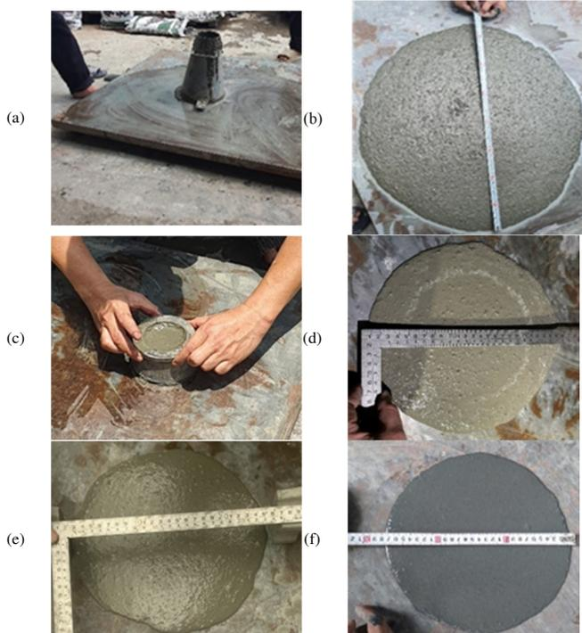
Fig. 9. (a) Slump flow (mini-slump cone), (b) slump flow of UHPC, (c) slump flow test (C230 cone), (d) slump flow of 100% CS, (e) slump flow of 50% CS, (f) slump flow of 0% CS-100% SS.
