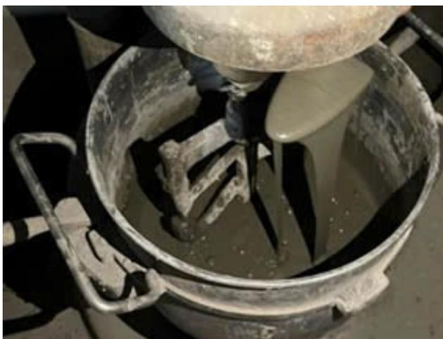
Fig. 5. Four-level forced mixing equipment.
