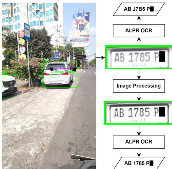
Fig. 3. The plate number detection with and without image processing.
